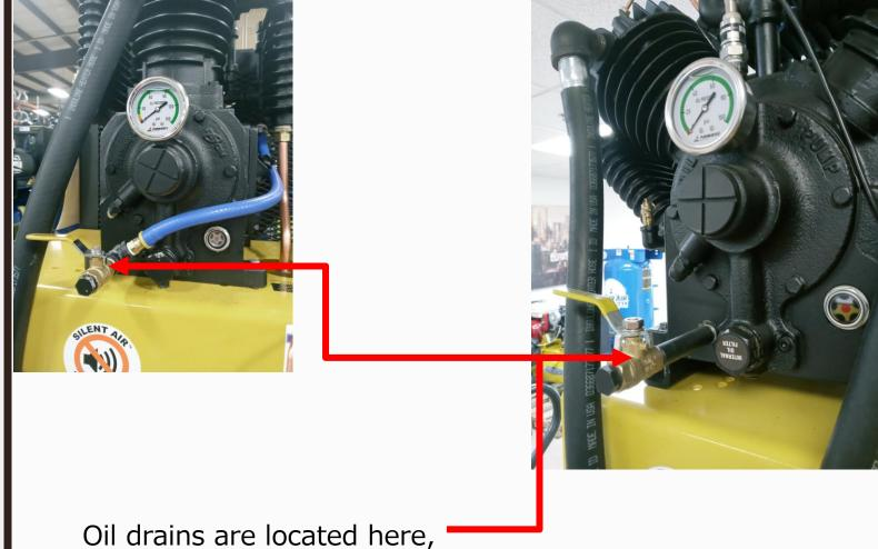
Oil drains are located here, Remove the end cap and open the ball valve. Once opened the oil will begin to flow out so have a catch can ready.
